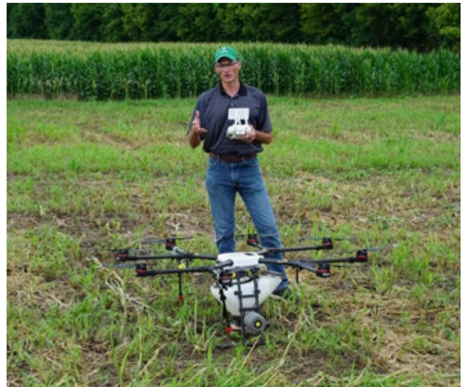
Figure 11. Top: Sugar Creek Valley Farms modified corn planter. Middle: Roller-crimper displayed at Virtual Field Day. Bottom: Rantizo drone equipped to broadcast cover crop seed.
